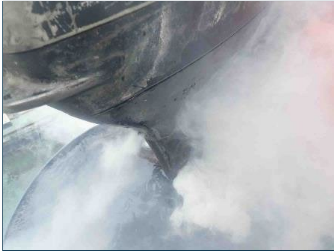
Outboard motor cooling system not functioning
