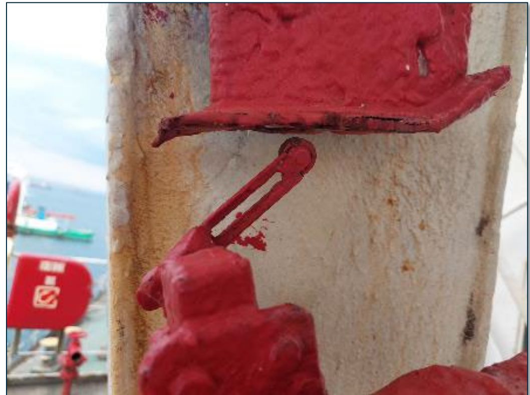
Defective / seized limit switches
