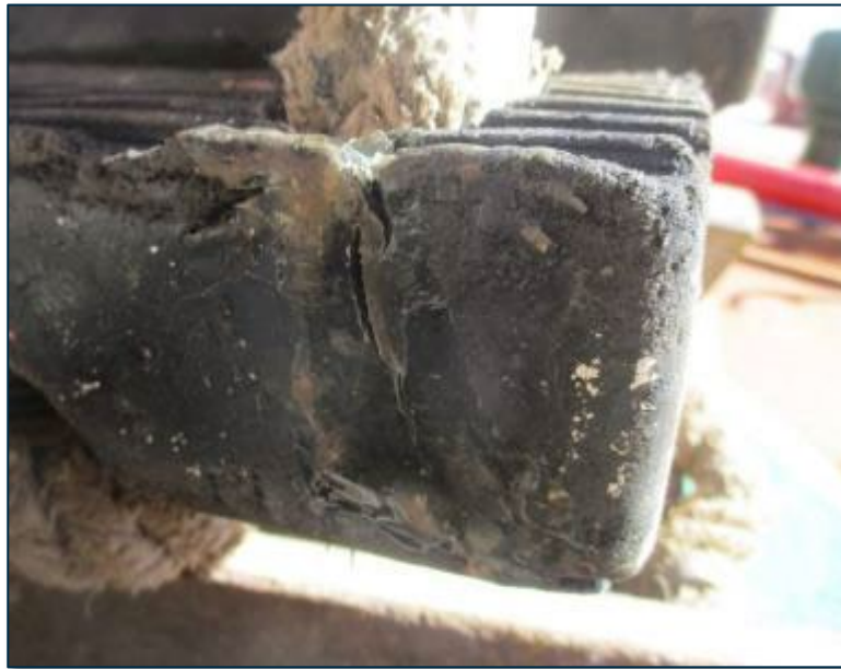
Pilot ladder rubber steps damaged
