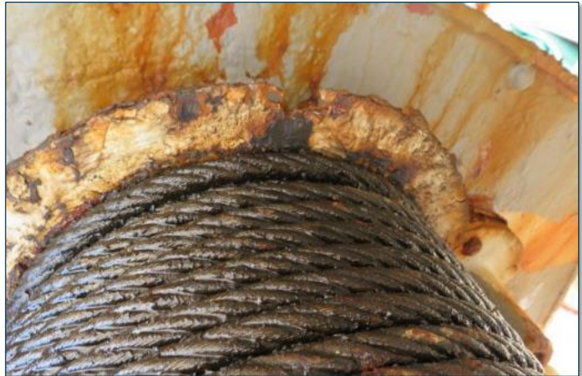
Lifeboat winch drums corroded
