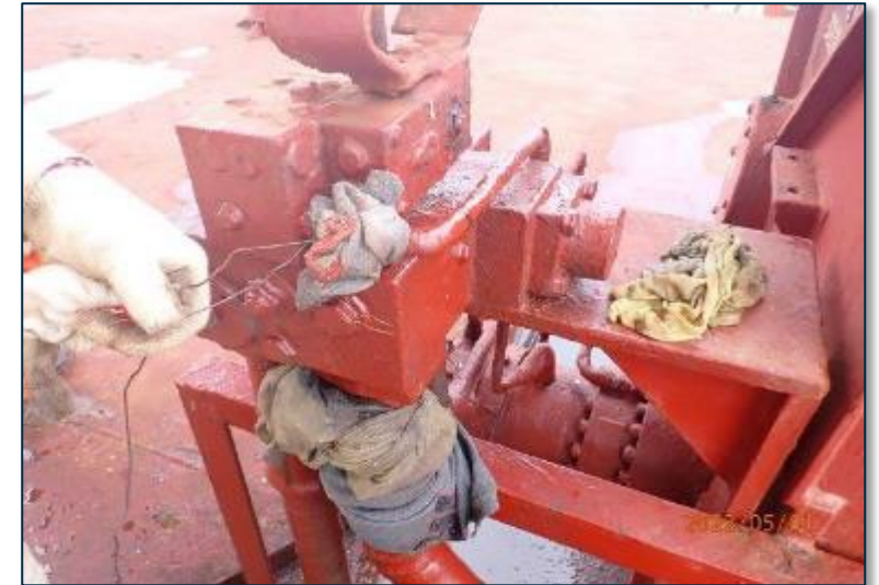
Hydraulic leaks from winches and windlasses
