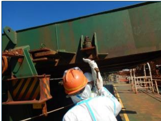
Seized / damaged securing cleats
