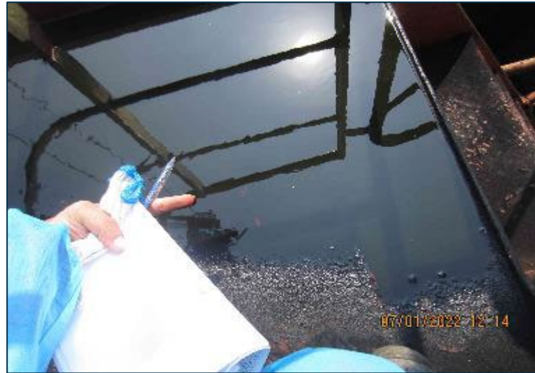
Hydraulic leaks from winches and windlasses
