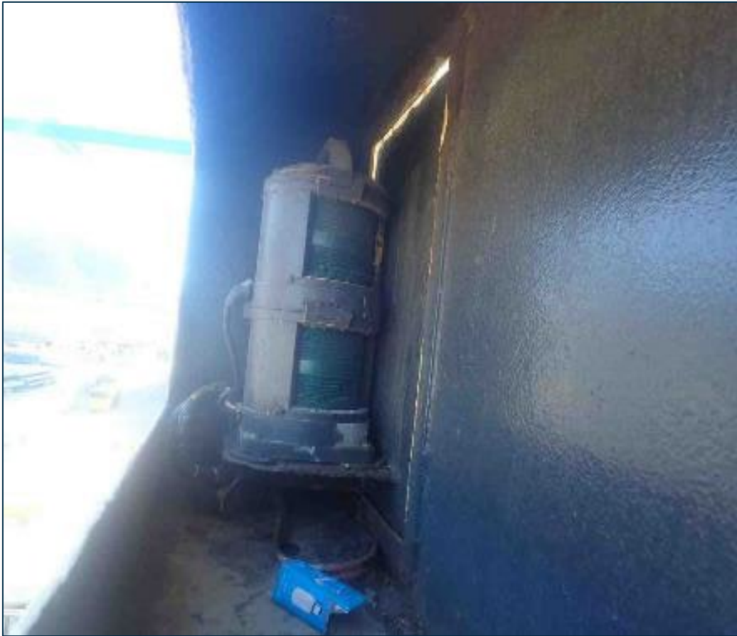
Starboard side light is mounted in the opposite way
