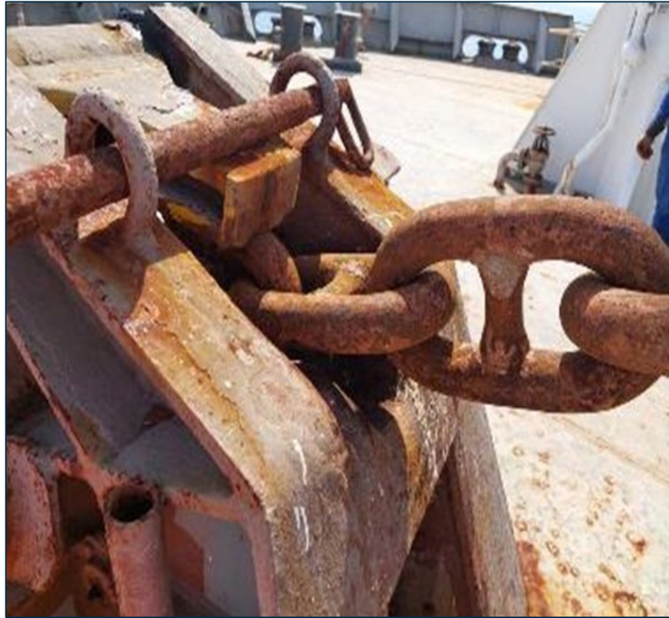
Chain not resting on stopper at anchor home position
