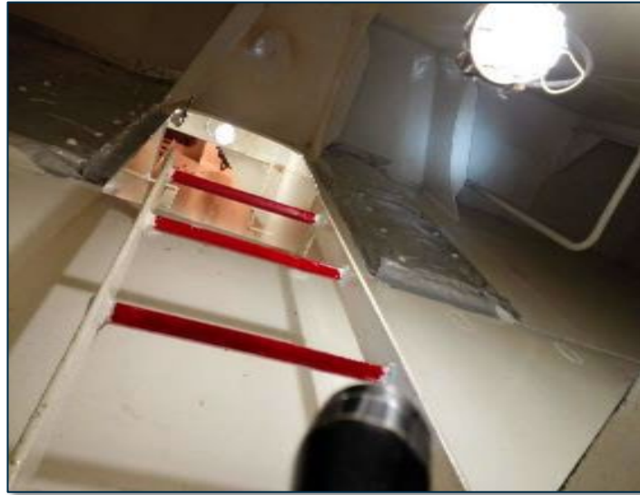
Escape trunk insulation missing
