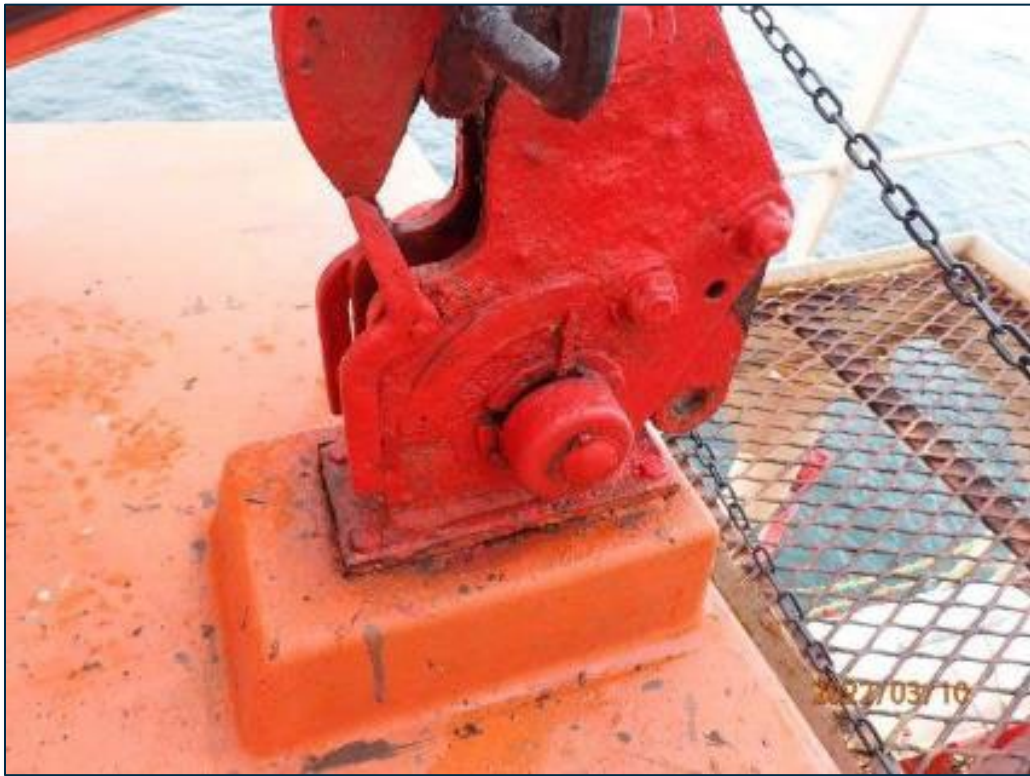
Lifeboat hooks painted covering lock indicators
