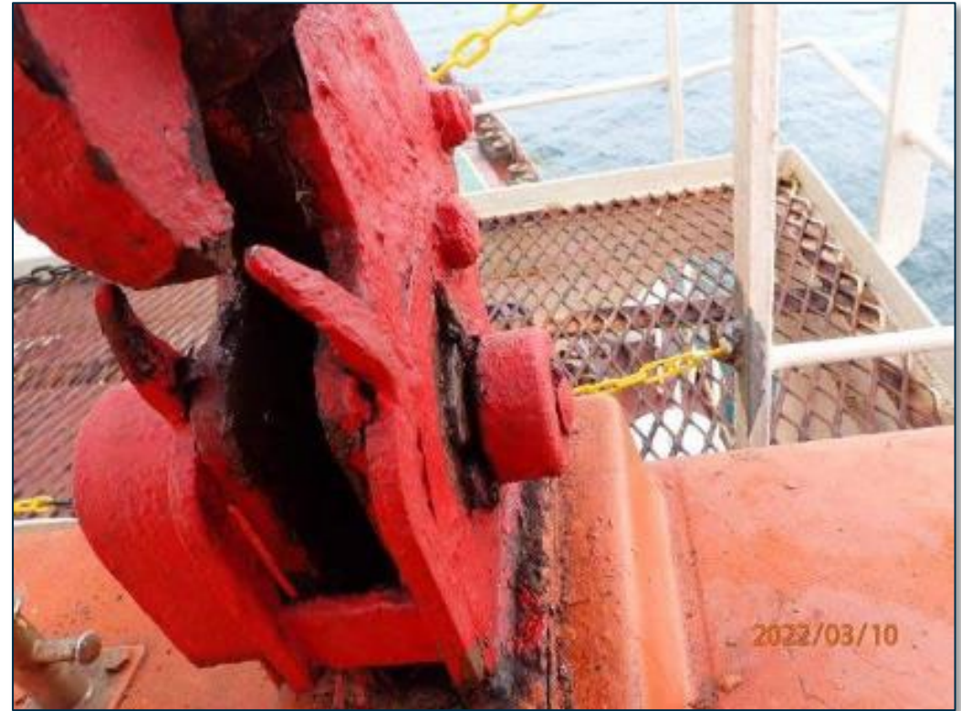
Lifeboat hooks painted covering lock indicators
