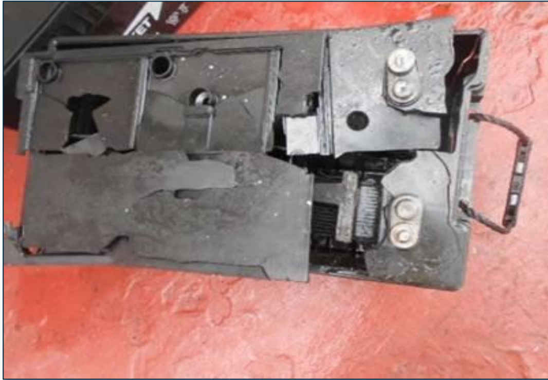
Emergency generator batteries explosion during testing
