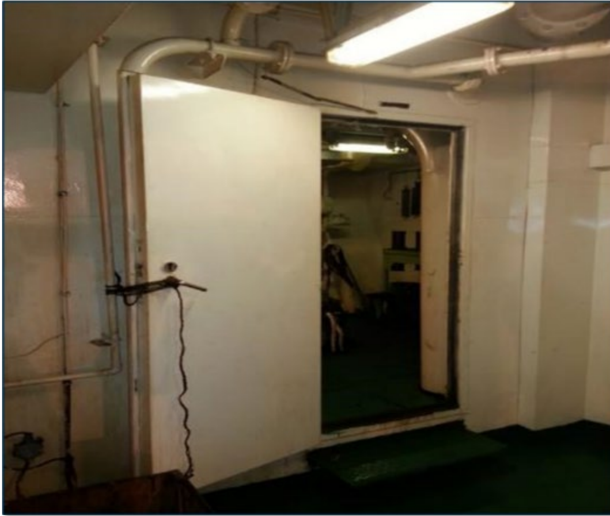
Class A door secured open
