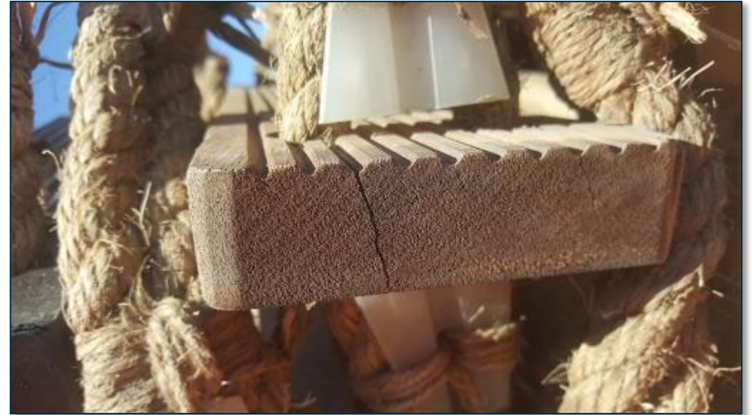
Pilot ladder wastages and cracks
