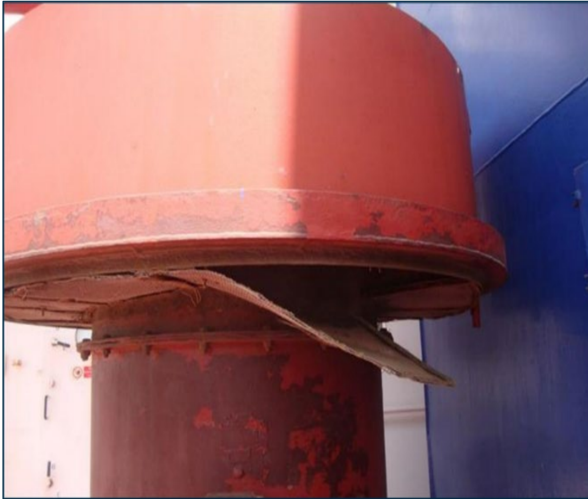
Main engine vent fan wire mesh in poor condition
