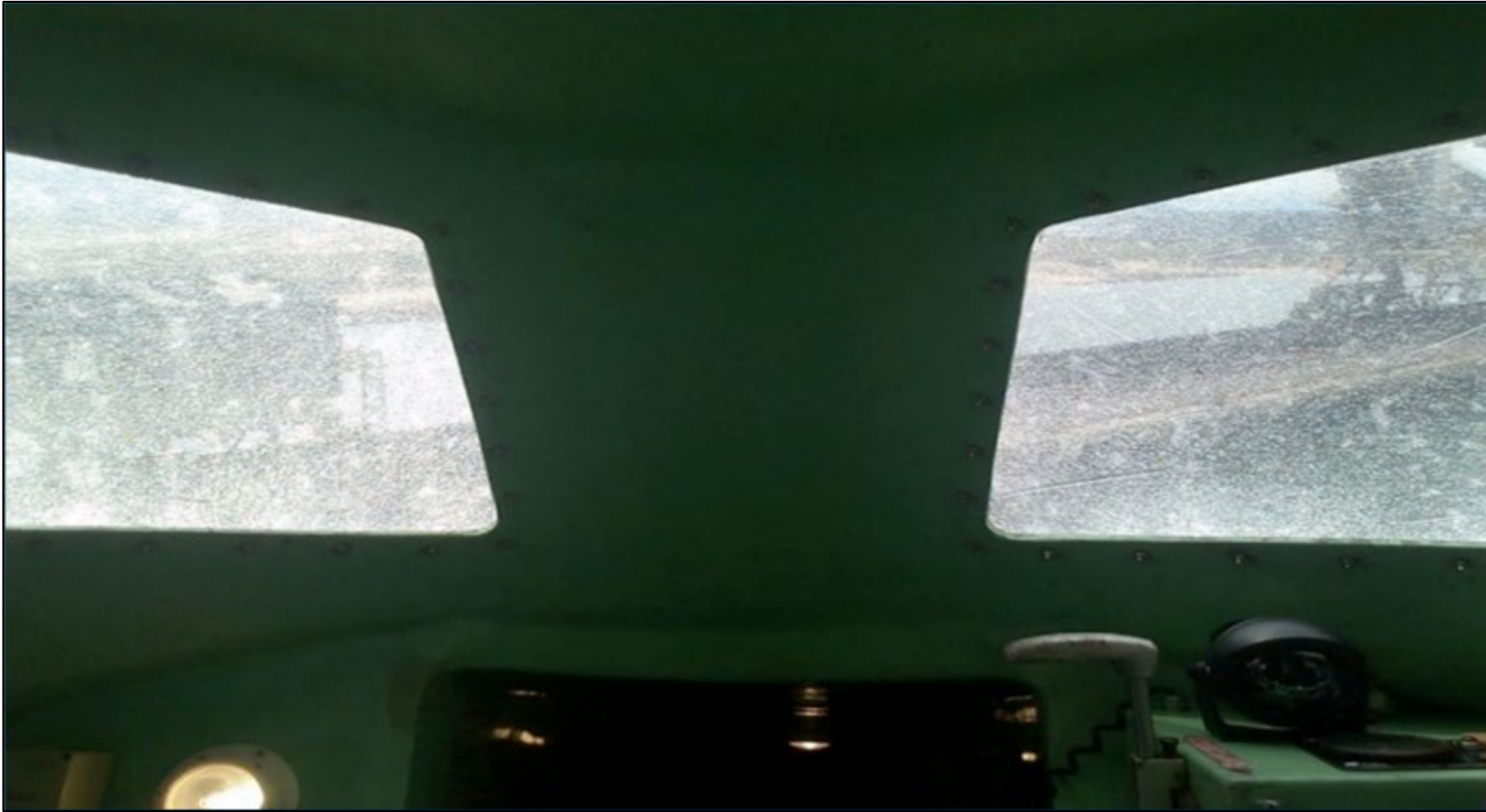
Free fall (FF) lifeboat front glass is obscured or opaque
