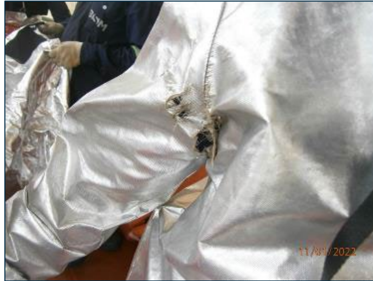
Damaged firefighter's outfit
